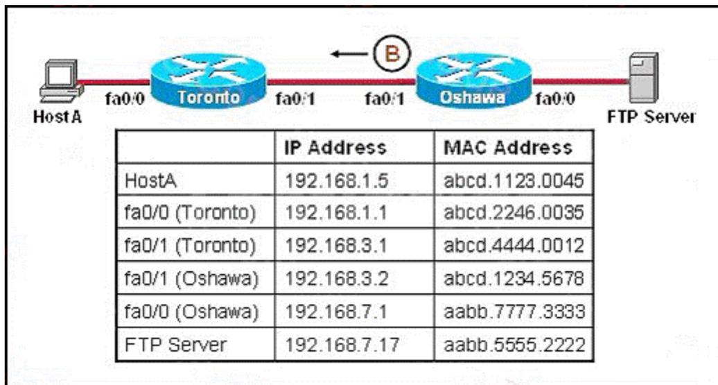
HostB is sending a file to HostA. B represents the frame as it leaves the Oshawa router. What is the Layer 2 destination address of the frame at this point?
