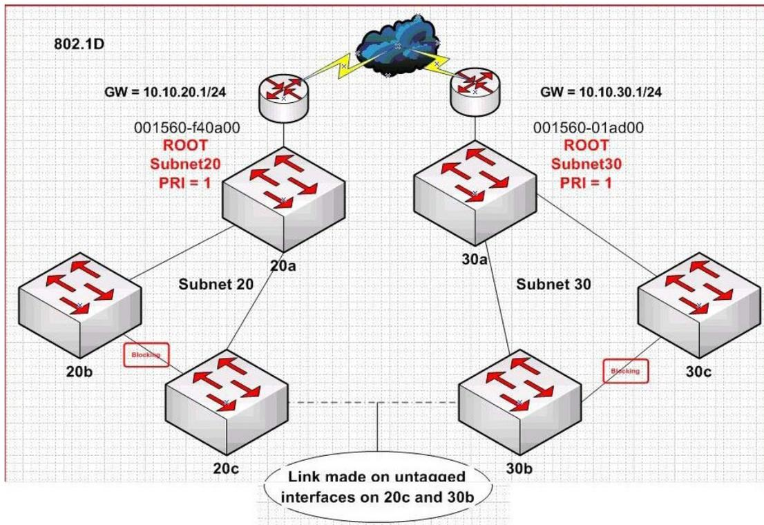
A user adds an untagged link between switch 20c and 30b. What is the impact of the user's actions?
