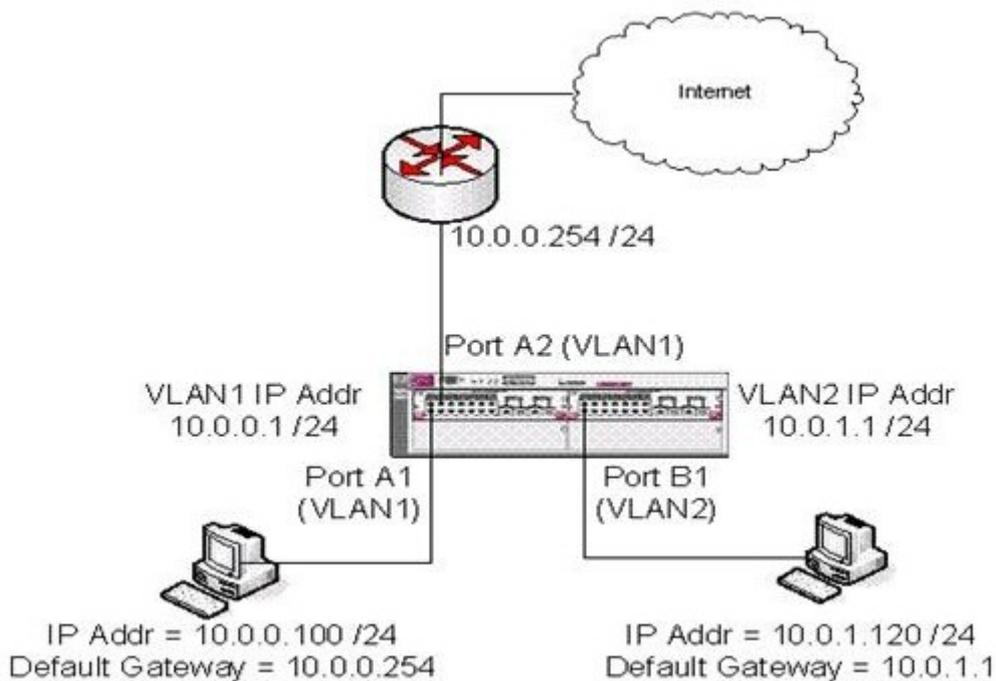
You need to limit the amount of broadcast traffic in this customer's network. In order to do so, you add a second VLAN, VLAN2 (10.0.1.0/24). Now, clients on VLAN2 cannot reach the Internet and cannot ping clients on VLAN1. They can successfully ping the default gateway (10.0.1.1). What should you do first to determine the cause of the problem?
